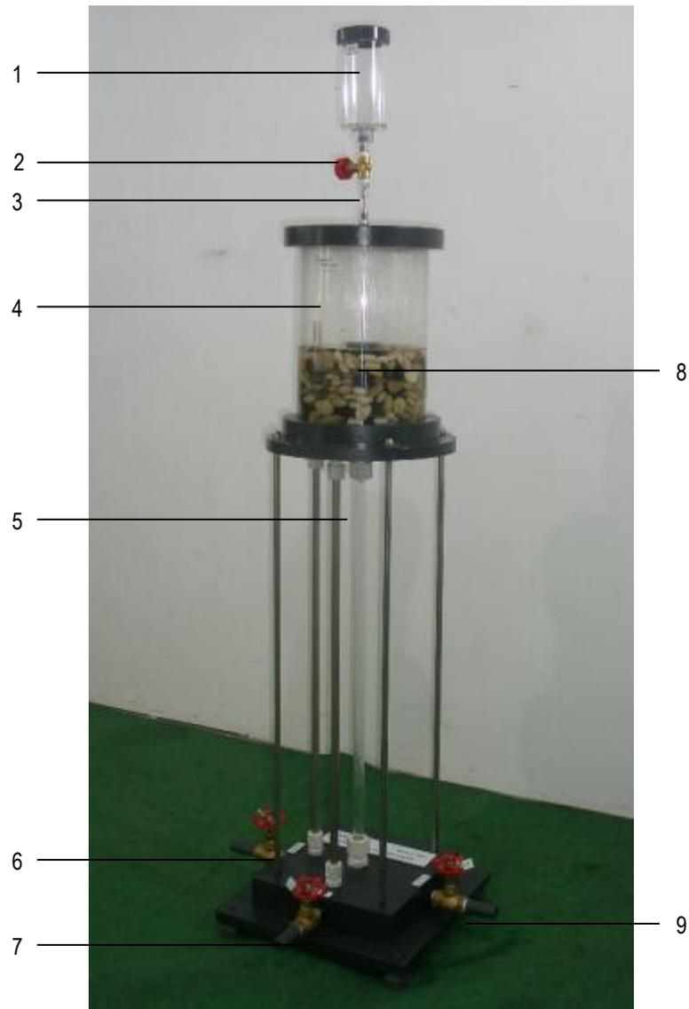
**Figure 1:** Unit Assembly of Osborne Reynolds Demonstration (Model: FM11)
