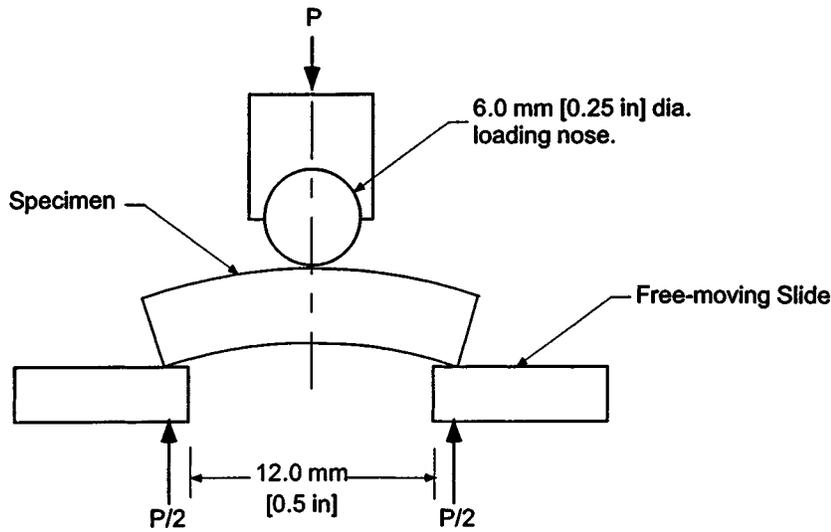
FIG. 5 Horizontal Shear Load Diagram (Curved Beam)
