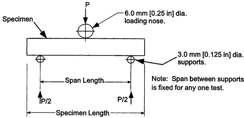
FIG. 6 Horizontal Shear Load Diagram (Flat Laminate)
