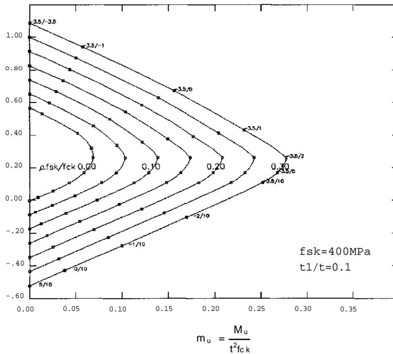
Fig. 8: Dimensioning Diagram for the Determination of the Ratio of Reinforcement  $p$  and the Wall Thickness  $t$  of Rectangular Cross-sections with  $t_1/t = 0.10$
