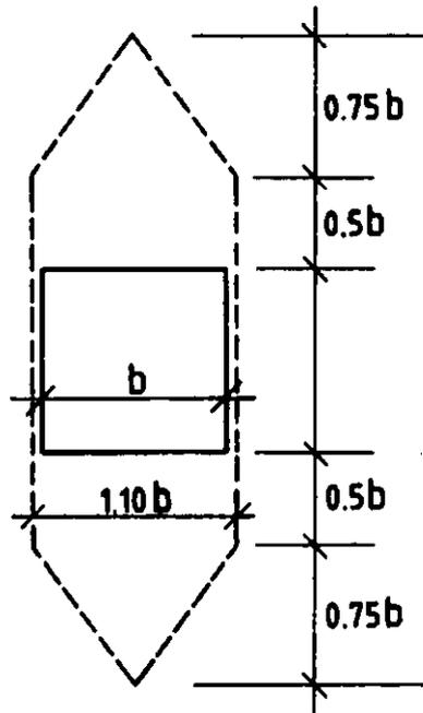
Figure 2 - Relation of real opening (solid line) to virtual opening (dashed line)
