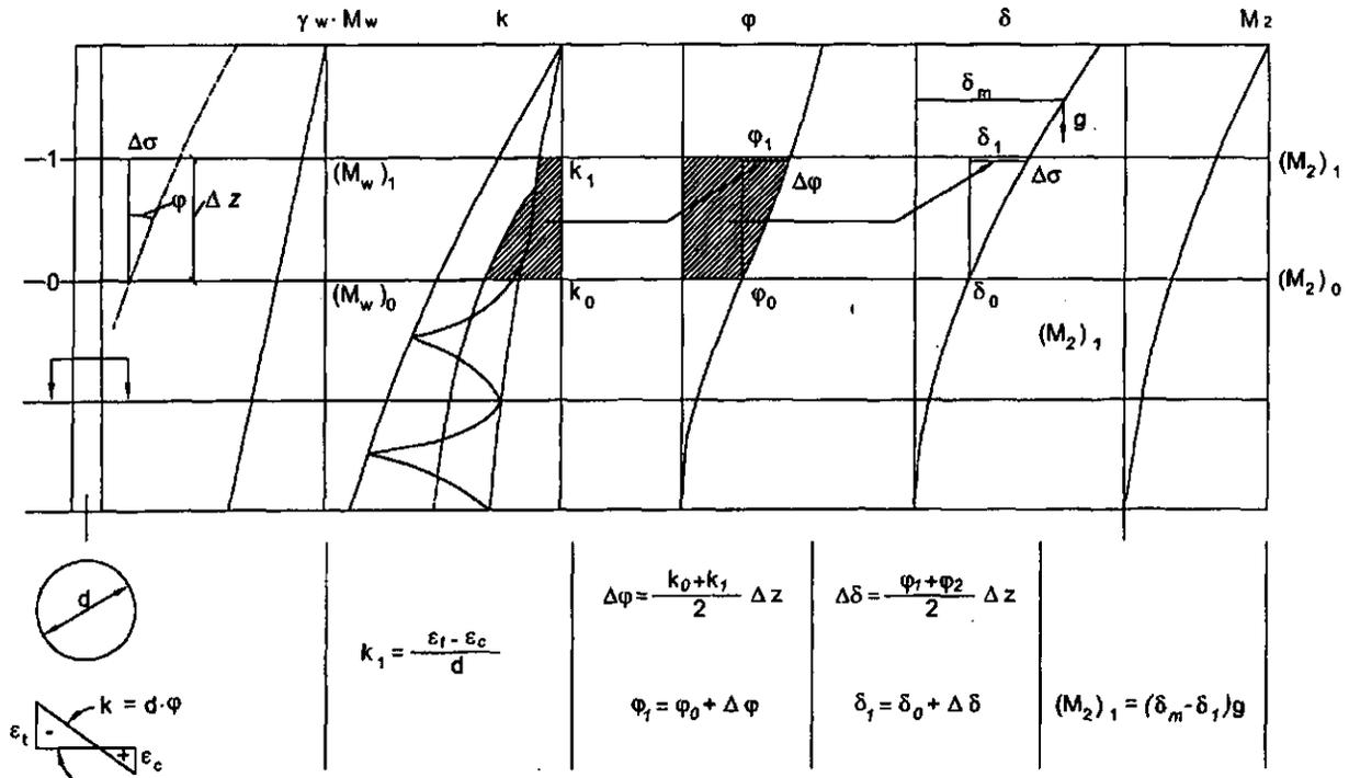
**Figure 4 :** Procedure for the exact determination of deflections and moment of 2<sup>nd</sup> order  $M_2$  according to Ref. 3
