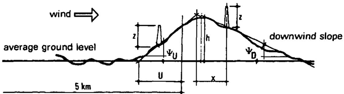
Figure 7 - Hill parameters for determining  $k_t$
