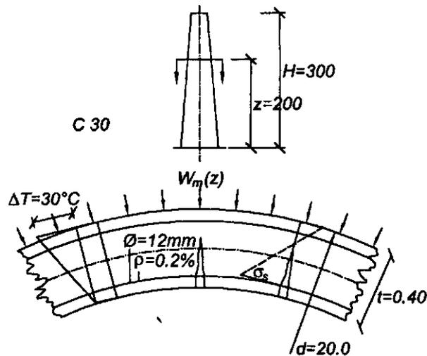
**Figure 6** : Cross-section of a chimney with circumferential reinforcement: Example for explanation
