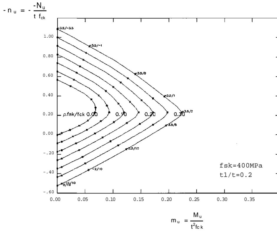
Fig. 9: Dimensioning Diagram for the Determination of the Ratio of Reinforcement  $p$  and the Wall Thickness  $t$  of Rectangular Cross-sections with  $t_1/t = 0.20$
