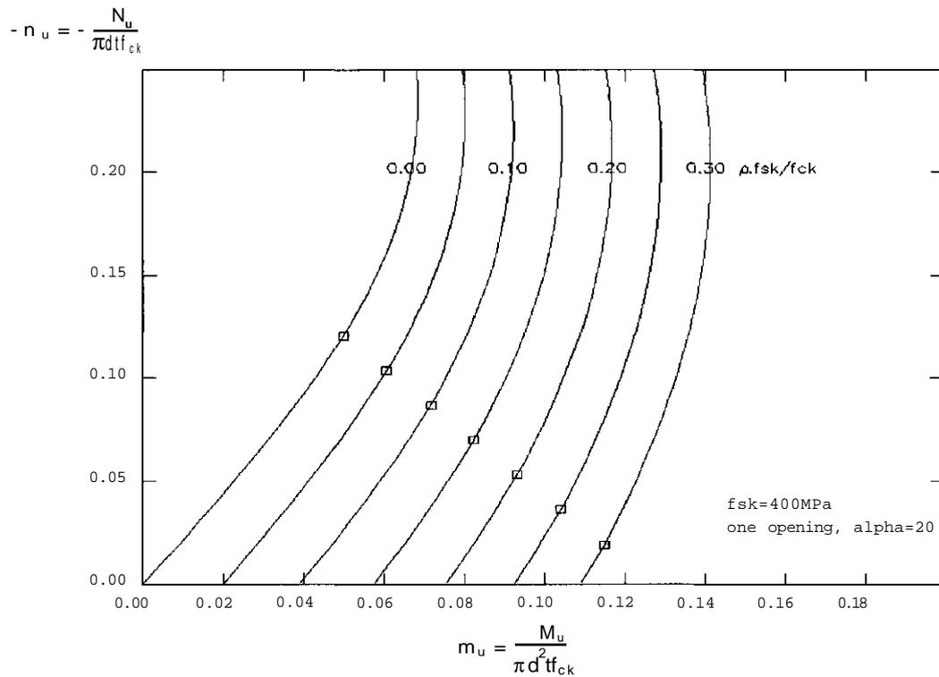
Fig. 3: Dimensioning Diagram for the Ratio of Reinforcement  $\rho$  and the wall thickness  $t$  of horizontal cross-sections with one opening of  $\alpha = 20^\circ$
