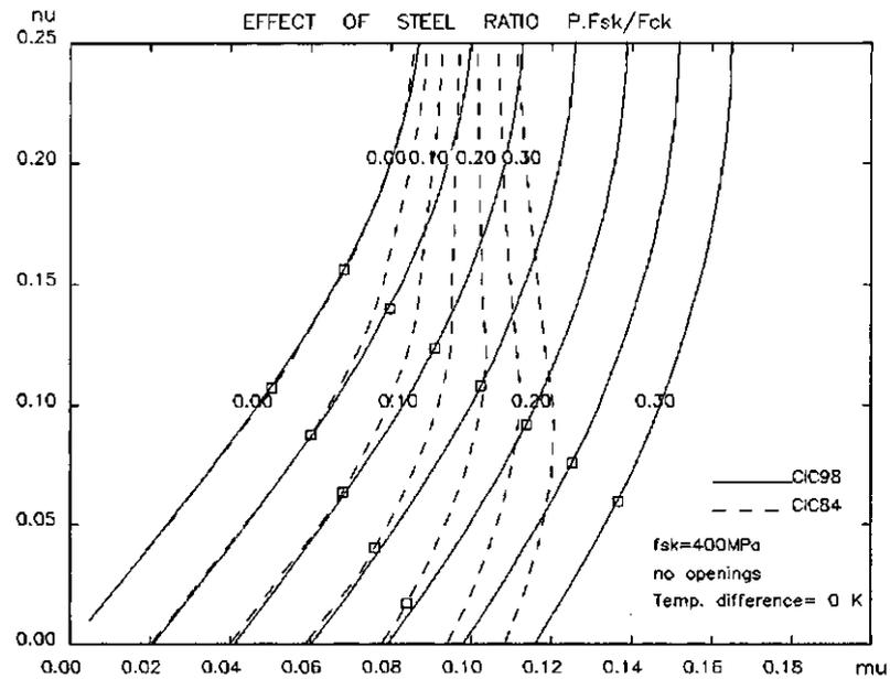
Fig. 1 - Comparison of design strengths for the old and new material laws - no openings
