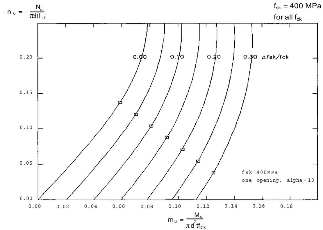
Fig. 2: Dimensioning Diagram for the Ratio of Reinforcement  $\rho$  and the wall thickness  $t$  of horizontal cross-sections with one opening of  $\alpha = 10^\circ$
