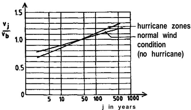
Figure 1 - Ratio between values of mean wind speed  $v_j$  with a return period of  $j$  years and the Basic Win Speed  $v_b$  with a return period of 50 years
