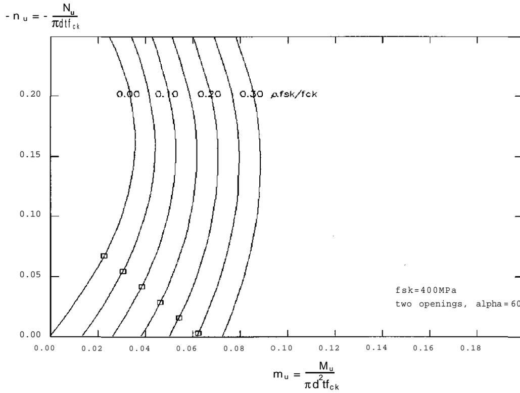
Fig. 13: Dimensioning Diagram for the Ratio of Reinforcement  $\rho$  and the wall thickness  $t$  of horizontal cross-sections with two opposed openings of  $\alpha = 60^\circ$
