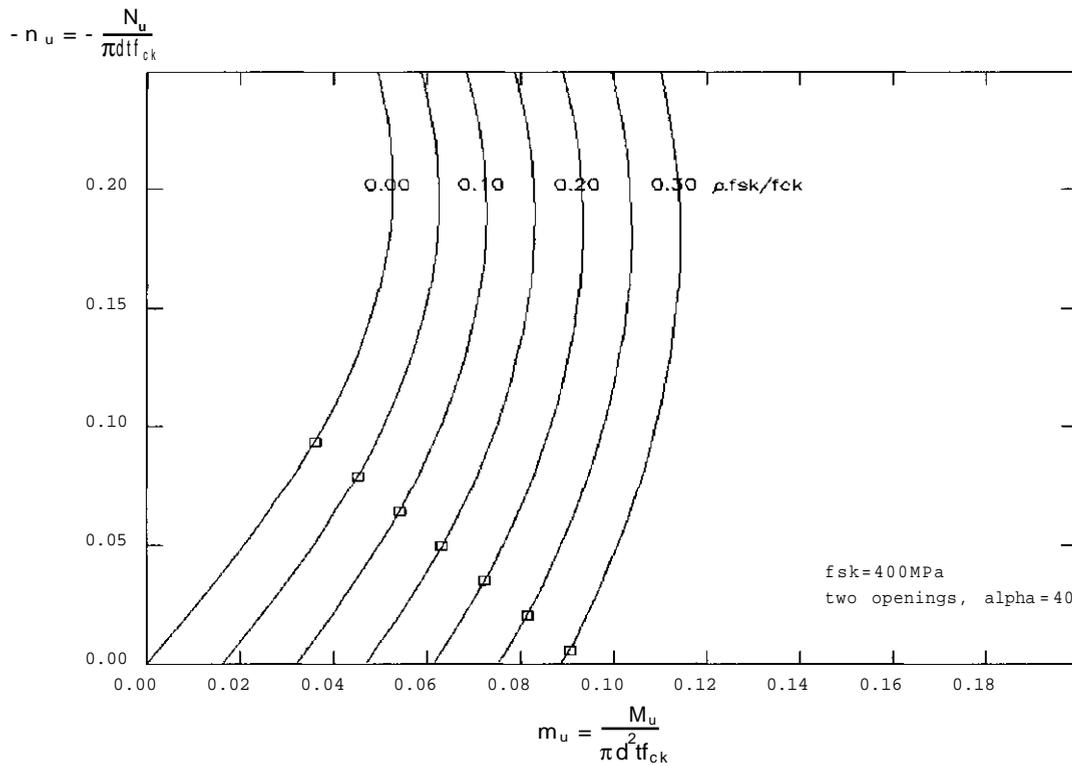
Fig. 11: Dimensioning Diagram for the Ratio of Reinforcement  $\rho$  and the wall thickness  $t$  of horizontal cross-sections with two opposed openings of  $\alpha = 40^\circ$
