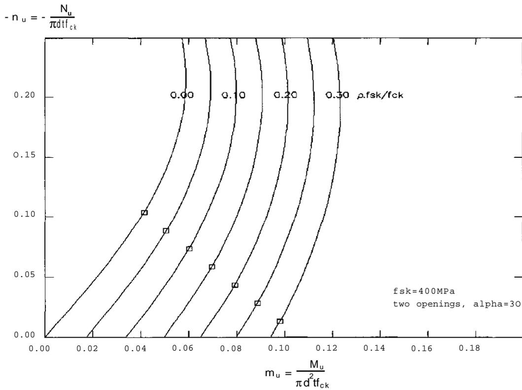
Fig. 10: Dimensioning Diagram for the Ratio of Reinforcement  $\rho$  and the wall thickness  $t$  of horizontal cross-sections with two opposed openings of  $\alpha = 30^\circ$
