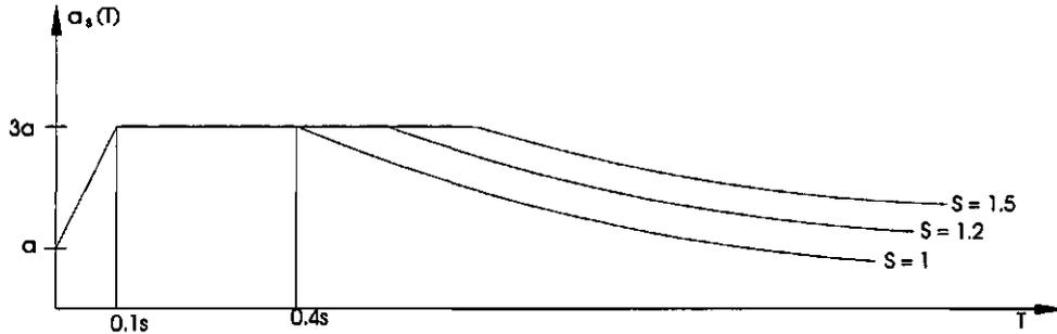
Figure 1 Response spectra for different soil types
