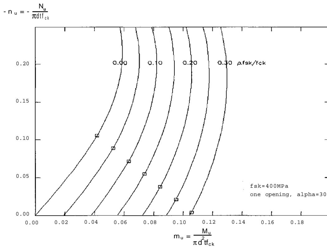
Fig. 4: Dimensioning Diagram for the Ratio of Reinforcement  $\rho$  and the wall thickness  $t$  of horizontal cross-sections with one opening of  $\alpha = 30^\circ$
