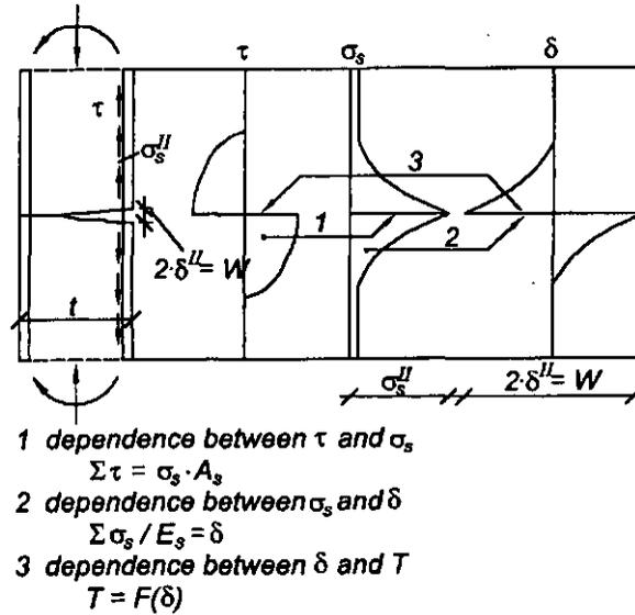
Figure 5 : Relations for the determination of the crack width
