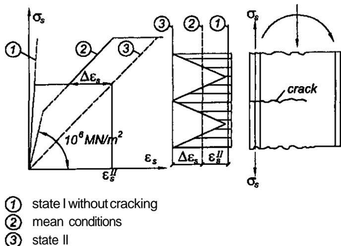
**Figure 1 :** Explanation of the Tension Stiffening Effect
