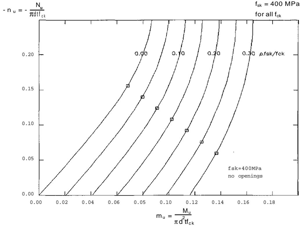
Fig. 1: Dimensioning Diagram for the Ratio of Reinforcement  $\rho$  and the wall thickness  $t$  of horizontal cross-sections with no openings
