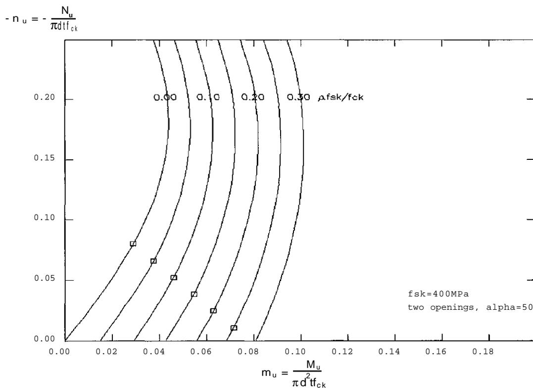
Fig. 12: Dimensioning Diagram for the Ratio of Reinforcement  $\rho$  and the wall thickness  $t$  of horizontal cross-sections with two opposed openings of  $\alpha = 50^\circ$
