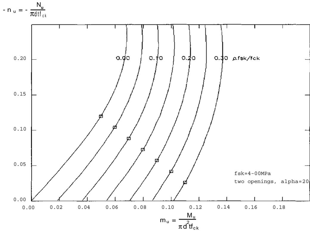
Fig. 9: Dimensioning Diagram for the Ratio of Reinforcement  $\rho$  and the wall thickness  $t$  of horizontal cross-sections with two opposed openings of  $\alpha = 20^\circ$
