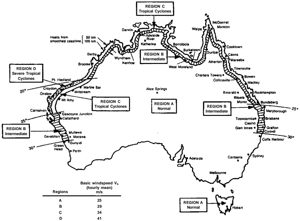
Figure 6 - Basic wind speeds  $v_b$  in m/s for Australia according to [3] (10m above ground, open country, 50 years return period, hourly mean).
