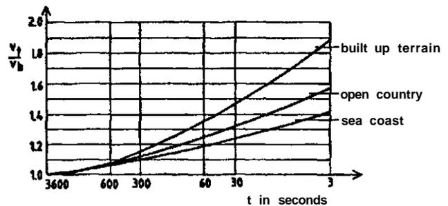
Figure 2 - Ratio between wind speeds  $v_t$  with averaging time  $t$  and the hourly Basic Wind Speed  $v_b$  as a function of averaging time
