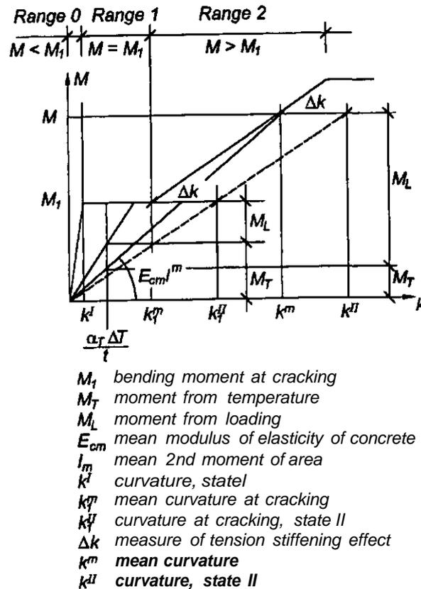
Figure 4 : Moment curvature relation of the considered bar divided into three ranges of crack formation
