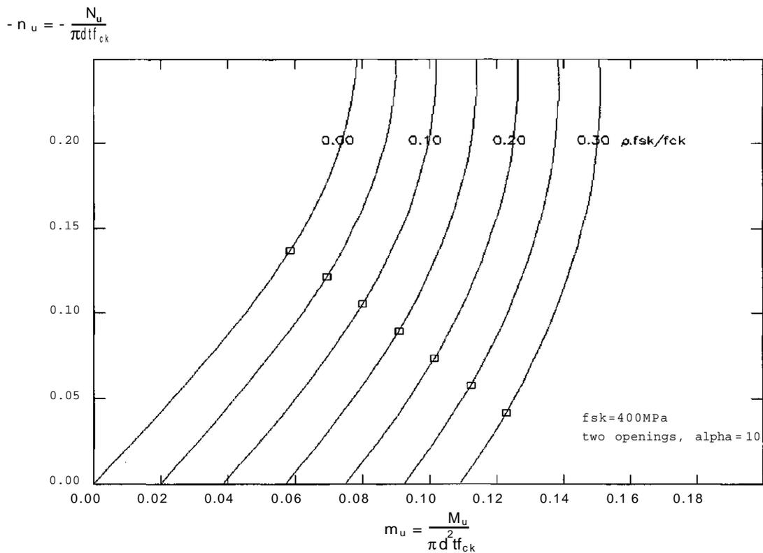
Fig. 8: Dimensioning Diagram for the Ratio of Reinforcement  $\rho$  and the wall thickness  $t$  of horizontal cross-sections with two opposed openings of  $\alpha = 10^\circ$
