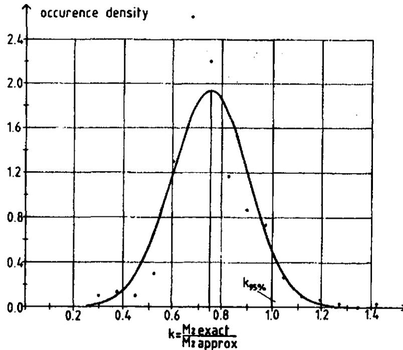
**Figure 5** : Occurrence density of ratios of exact moment of 2<sup>nd</sup> order to approximate moment of 2<sup>nd</sup> order for 60m representative chimneys with 5 cross-sections per chimney
