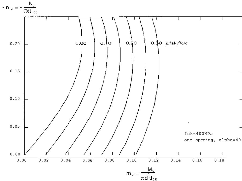
Fig. 5: Dimensioning Diagram for the Ratio of Reinforcement  $\rho$  and the wall thickness  $t$  of horizontal cross-sections with one opening of  $\alpha = 40^\circ$
