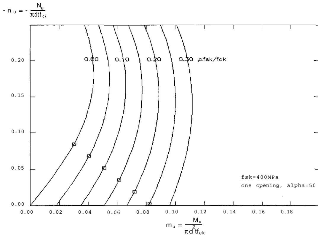
Fig. 6: Dimensioning Diagram for the Ratio of Reinforcement  $\rho$  and the wall thickness  $t$  of horizontal cross-sections with one opening of  $\alpha = 50^\circ$
