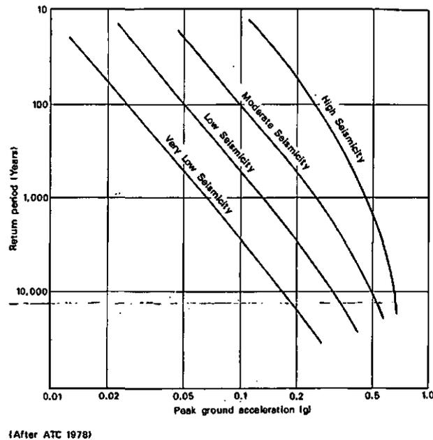
**Figure 3 - Peak ground acceleration as a function of return period and seismicity****4 References**
