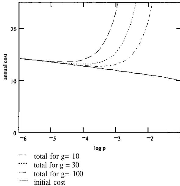
**Fig.1 Total Cost vs. Failure Probability**
