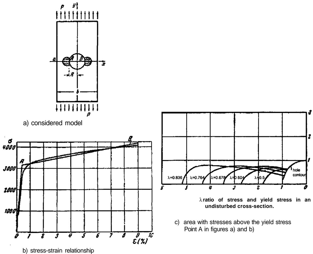
Figure 3 - Material plastification next to openings according to [1]
