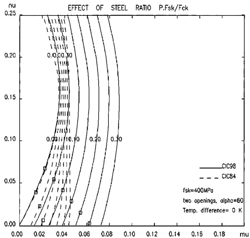
Fig.2 - Comparison of design strengths for the old and new material laws - two opposed openings
