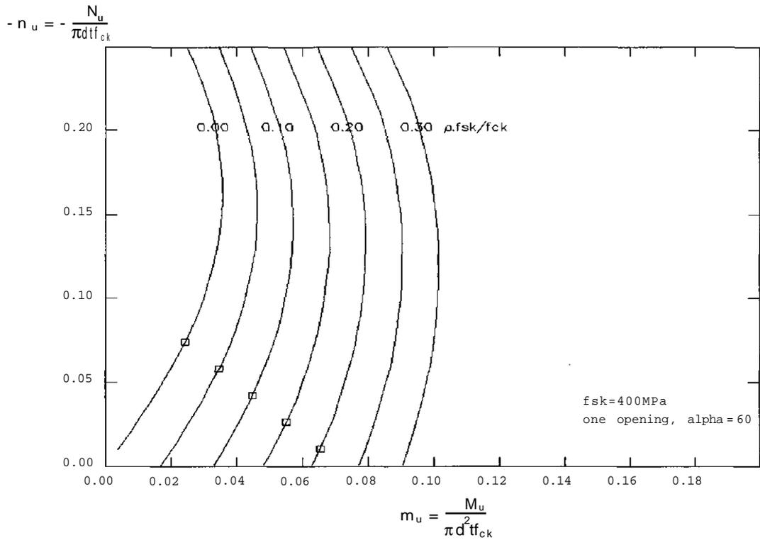
Fig. 7: Dimensioning Diagram for the Ratio of Reinforcement  $\rho$  and the wall thickness  $t$  of horizontal cross-sections with one opening of  $\alpha = 60^\circ$
