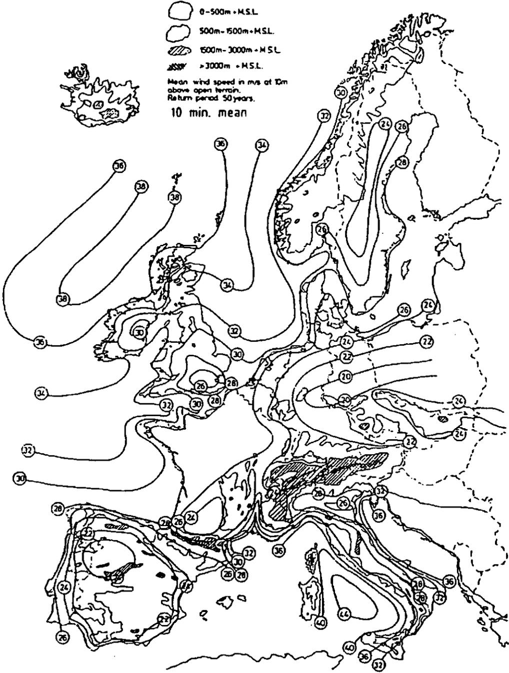
Figure 3 - Basic wind speeds  $v_b$  in m/s for Europe according to [1] (10m above ground, open country, 50 years return period)
