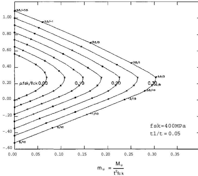
Fig. 7: Dimensioning Diagram for the Determination of the Ratio of Reinforcement  $p$  and the Wall Thickness  $t$  of Rectangular Cross-sections with  $t_1/t = 0.05$
