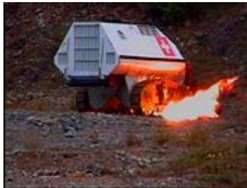
Digger D1 tested with a charge of TNT
