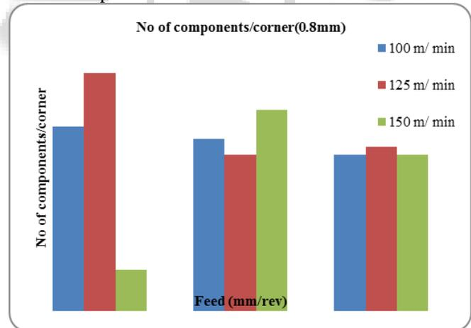
Fig. 2: Feed vs Number of components/corner
