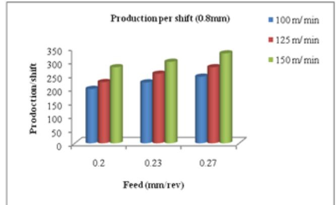
Fig. 4: Feed vs Production/shift
