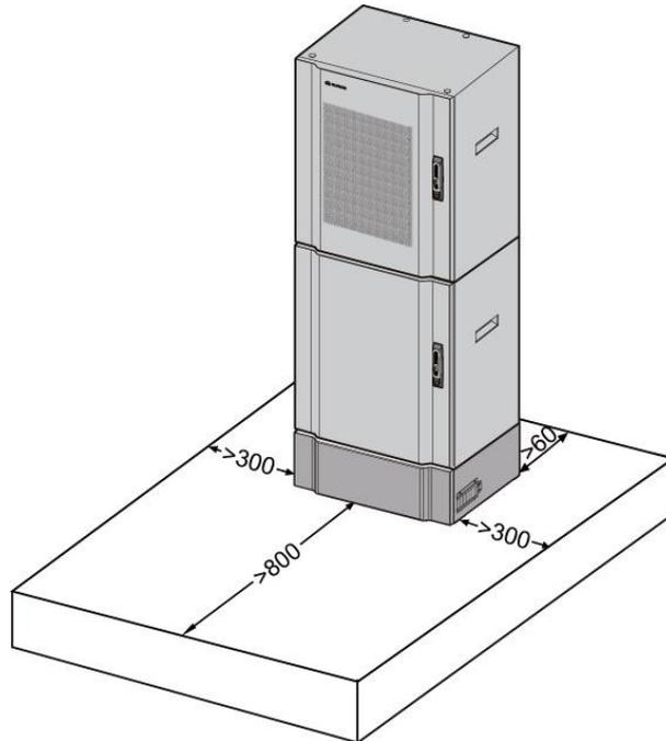
Space requirements for installing the BTS3900A configured with the RF cabinet, power cabinet, and extension cabinet (unit: mm)
