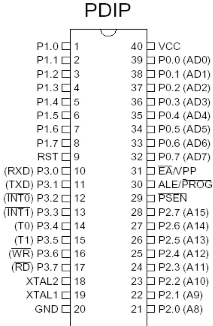
**Fig: Pin Configuration of AT89C51**
