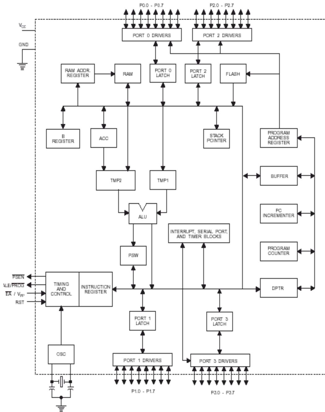
**Fig: Block Diagram of AT89C51 Microcontroller**
