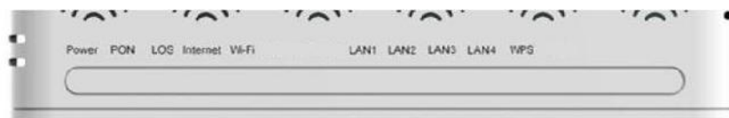
Figure 3-2 LED Indicators of the ZXHN F600W
