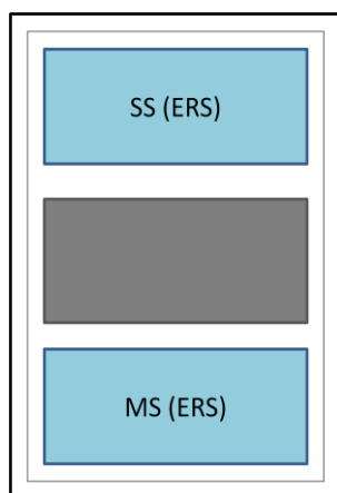
Figure 5-5 Large Capacity Configuration within Two Shelves of ZXUR 9000 UMTS
