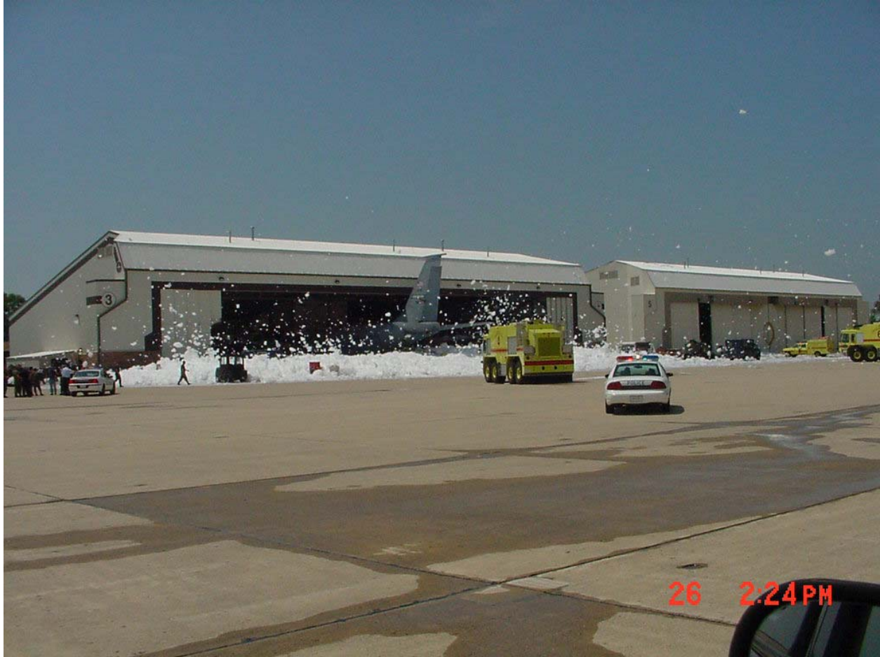
Figure A2.5. Low-Level High-Expansion Foam After 7-Minute Discharge
